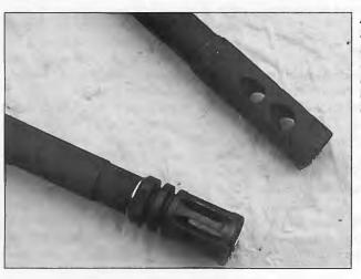
As opposed to a standard flash hider, the Bushmaster M4 Type Carbine comes with a Mini Y Muzzle Brake that is an integral part of the barrel.
